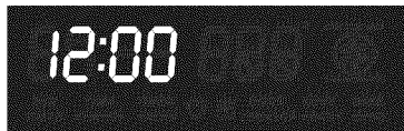
Fig. 28 12:00 displayed when oven is powered up or power is restored after an interruption
