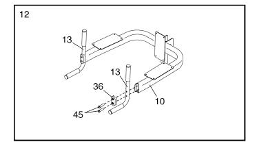
Attach an Armrest (16) to the Dip Arm (10) with four M6 x 20mm Screws (41). Start all four Screws, and then tighten them.
