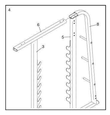
Attach the Top Frame (6) to the Right Rear Frame (8) and to the Right Center Upright (5) with two M10 x 75mm Screws (43), two M10 Washers (37), and two Frame Spacers (29); do not tighten the Screws yet.
