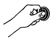
Line up openings in the reflector bowl with the surface unit receptacle and the element holddown clip.
