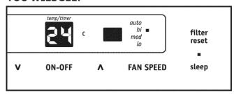
Note: In this mode the selected temperature will increase by 1 °C 30 minutes after the mode is selected. The temperature will then increase by another 1 °C after an additional 30 minutes. This new temperature will be maintained for 7 hours before it returns to the originally selected temperature. This ends the "Sleep" mode and the unit will continue to operate as originally programmed. The "Sleep" mode program can be cancelled at any time during operation by again pressing the "Sleep" button.
