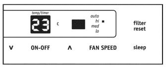
Note: Tap or hold either up (  $\Lambda$  ) or down ( V ) button until the desired temperature is seen on the display. This temperature will be automatically maintained anywhere between 16 °C (60 °F) and 32 °C (90 °F) . If you want the display to read the actual room temperature. See "To Operate on Fan Only" section on Page 7.
