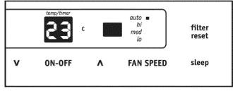
Note: Fan starts at High Speed and adjusts to a slower speeds the room temperature dictates. For example, if the room doesn't get too warm, it will stay at the slowest speed. If the room temperature rises quickly, such as a door being opened, it will automatically go to the highest speed. The fan speeds will re-adjust back to the slowest speed as the room returns to the original set temperature. Press either the fan slower or fan faster button to adjust the fan speed manually.
