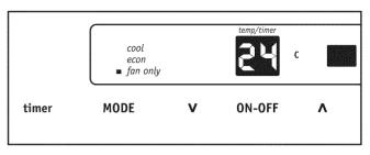
Note: Use this function only when cooling is not desired, such as for room air circulation or to exhaust stale air on some models. (Remember to open the vent during this function, but keep it closed during cooling for maximum cooling efficiency.) You can choose any fan speed you prefer. (Except "Auto Fan").
