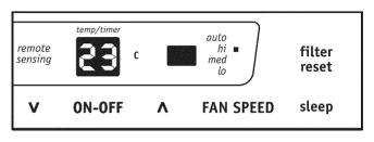
Note: Tap or hold either up (  $\Lambda$  ) or down ( V ) button until the desired temperature is seen on the display. This temperature will be automatically maintained anywhere between 16 °C (60 °F) and 32 °C (90 °F) . If you want the display to read the actual room temperature. See "To Operate on Fan Only" section on Page 7.
