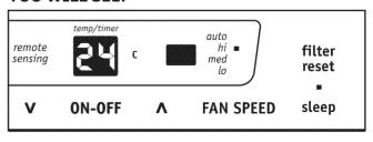
Note: In this mode the selected temperature will increase by 1 °C 30 minutes after the mode is selected. The temperature will then increase by another 1 °C after an additional 30 minutes. This new temperature will be maintained for 7 hours before it returns to the originally selected temperature. This ends the "Sleep" mode and the unit will continue to operate as originally programmed. The "Sleep" mode program can be cancelled at any time during operation by again pressing the "Sleep" button.
