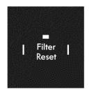
After 250 hours of operation, the Filter Reset LED will light. This is a reminder to clean the filter housed behind the front panel to keep the unit operating efficiently. Pressing the FILTER RESET button for 3 seconds will reset this reminder and turn off the LED.
