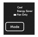
Use Fan Only function to circulate room air without air conditioner cooling. You can use any fan speed you prefer and the actual room temperature will be displayed in the DISPLAY.
