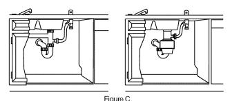
Method 2 – High Drain with Waste Tee or Disposer Provide a method to attach drain hose to underside of countertop.
