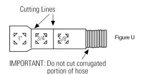
• If a longer drain hose is required, add up to 42" of length for a total of 10 ft. to the factory installed hose. Use 5/8" or 7/8" inside diameter hose and a coupler to connect the two hose ends. Secure the connection with hose clamps.
