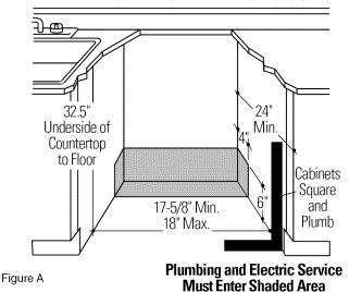
The rough cabinet opening must be at least 24" deep and 17-5/8" to 18" wide. The opening should be 32.5" max. height.
