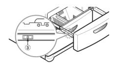
4 With the drawer pulled out to full extension, insert the basket and ice bin in the rail assembly.
