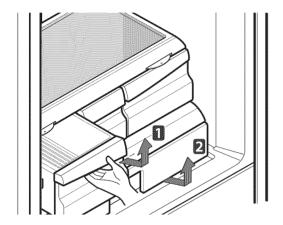
To install, slightly tilt up the front, insert the drawer into the frame and push it back into place.
