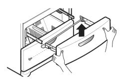
4 With both hands, hold each rail and push it in to allow both rails to slide in simultaneously.
