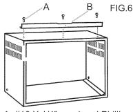
A. #10 X 1/4" pan-head Phillips thread cutting screwsB. Top channel
