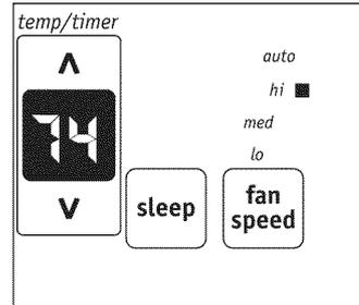
Note: Tap or hold either up ( ^ ) or down ( v ) button until the desired temperature is seen on the display. This temperature will be automatically maintained anywhere between 60 °F (16 °C) and 90 °F (32 °C) for cooling mode. The temperature will be automatically maintained anywhere between 55 °F (13 °C) and 80 °F (27 °C) for heating mode. If you want the display to read the actual room temperature. See "To Operate on Fan Only" section on Page 7.
