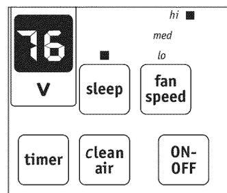
Note: In this mode the selected temperature will increase by 2 °F 30 minutes after the mode is selected. The temperature will then increase by another 2 °F after an additional 30 minutes. This new temperature will be maintained for 7 hours before it returns to the originally selected temperature. This ends the "Sleep" mode and the unit will continue to operate as originally programmed. The "Sleep" mode program can be cancelled at any time during operation by again pressing the "Sleep" button.
