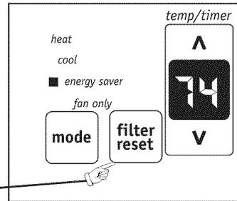
Note: This feature is a reminder to clean the Air Filter (See Care and Cleaning) for more efficient operation. The LED (light) will illuminate after 250 hours of operation. To reset after cleaning the filter, press the "Filter Reset" button and the light will go off.
