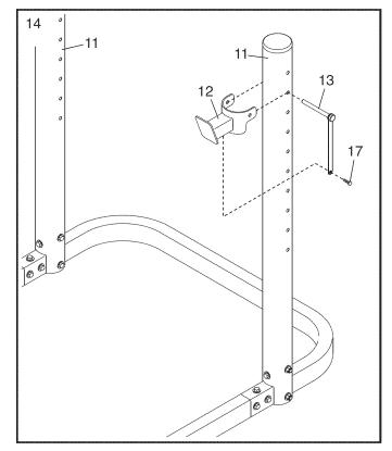
15. Attach the tether on a Large Pin (13) to the underside of a Spotter (29) with an ST4.2 x 16mm Screw (17).
