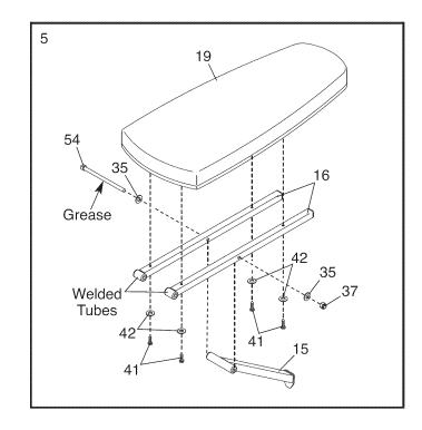
Apply a small amount of grease to an M10 x 192mm Bolt (43). Attach the Backrest Frames (16) to the Frame (1) with the Bolt, two M10 Washers (35), and an M10 Locknut (37). Do not overtighten the Locknut; the Backrest Frames should pivot easily.
