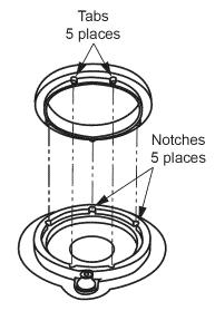
**Burner Ring Installation Detail**
