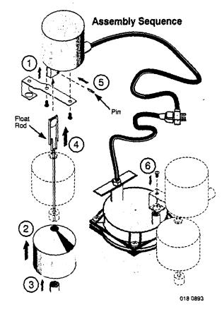
A CAUTION A CAUTION Make sure pin holds float rod in switch housing; otherwise pump will not shut off.
