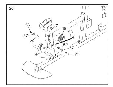
21. Route the Low Cable (53) through the Upright (3) and under a Thick Pulley (48).
