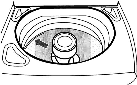
3. Pour measured liquid chlorine bleach into the liquid chlorine bleach dispenser, if needed. Bleach is fed into the washer and is diluted automatically during the wash cycle.
