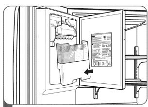
To reinstall the in-door ice bin, slightly slant the bin during replacement to avoid contact with the icemaker.
