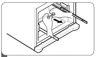
To reinstall the freezer drawer, place the bar back on edge of the gears in the secure holes on the opposite rails and pull out until the drawer rails are fully extended.
