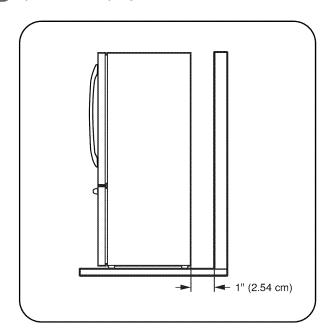
Too small a distance from adjacent items may result in lowered freezing capability and increased electricity consumption charges.
