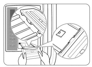
The dispenser drip tray has no self-draining function. It should be cleaned regularly. Remove the cover by pressing and pulling the tray. Dry it with a cloth. To reinstall the tray, slightly tilt the front of the tray and snap the ribs into the holes.
