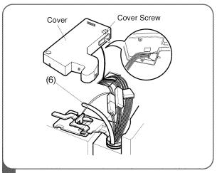
Push the water supply tube (6) into the hole on the top case and pull it through the backplate.
