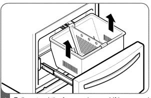
Fully extend the freezer drawer. Lifting up and out to remove the Dura Base basket making sure to clear the rail system.
