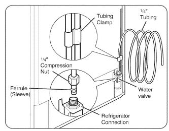
• Remove the plastic flexible cap from the water valve.
