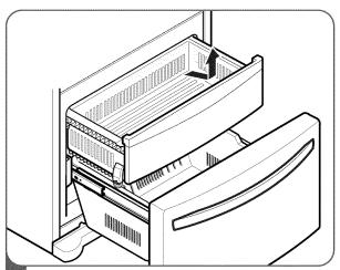
To remove the drawer, push the tabs located on the front inside surface of each rail. Next, gently lift the rear left and right sides of the drawer and pull it out.
