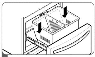
With the drawer pulled out to full extension, insert the lower basket in the rail assembly.
