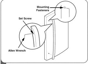
Loosen the set screws with a 2.5 mm (3/32") Allen wrench and remove the handle.
