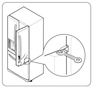
Use the wrench (Included with the User Manual) to adjust the bolt in the door hinge to adjust the height. (counter clockwise to raise or clockwise to lower)
