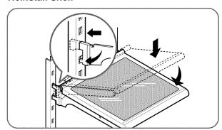
Tilt up the front of the shelf and guide the shelf hooks into the slots at a desired height. Then lower the front of the shelf so that the hooks drop into the slots.
