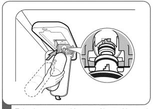
Take the new cartridge out of its packing and remove the protective cover from the o-rings. With cartridge ears in the horizontal position, push the new filter cartridge into the manifold hole until it stops.
