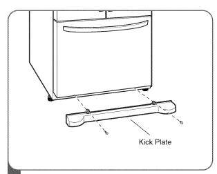
Plug the power cord into a 3-prong grounded outlet, and move the refrigerator into its final position. Remove the kick plate screws and then the kick plate.
