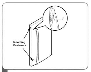
Place the handle on the door by aligning handle footprints to fit mounting fasteners and tighten the set screws with a 2.5 mm (3/32") Allen wrench.
