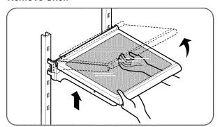
Tilt up the front of the shelf. Lift up the back and pull out the shelf.
