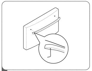
Place the handle on the door by aligning handle footprints to fit mounting fasteners and tighten the set screws on the bottom of the handle with a 3.1 mm (1/8") Allen wrench.
