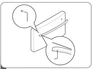
Loosen the set screws located on the lower side of the handle with a 3.1 mm (1/8") Allen wrench and remove the handle.
