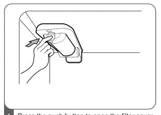
Press the push button to open the filter cover. **NOTE**: Replacing the filter causes a small amount of water (around 1 oz. or 25 cc) to
