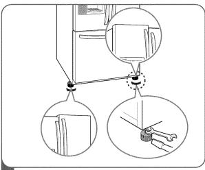
Level the refrigerator by using an 11/16 inch (18mm) wrench or a flat blade screw driver.
