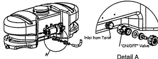
This unit comes with an On/Off valve, located near the inlet of the tank, towards the underside. (See Detail A)
