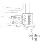
If the doors remain uneven, turn the adjustable pin to raise, or lower, the left door to match the right door. Use a 1/4 Allen wrench to turn the pin.
