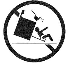
To reduce the risk of tipping, the range must be secured by properly installed anti-tip bracket provided with the range. To check if the bracket is installed properly, visually check that rear leveling leg is inserted into and fully secured by the anti-tip bracket by removing lower front panel or storage drawer from the range.
