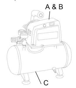
The pressure switch (located internally) shuts down the motor and relieves air pressure in the pump and transfer tube when the air pressure in the tank reaches the kick-out pressure. As compressed air is used and the pressure level in the tank drops to the kick-in pressure, the pressure, the pressure switch restarts the motor automatically, without warning, and the pump resumes compressing air.
