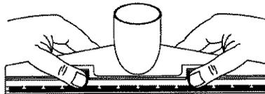
4. Inspect the pins of the insert to make sure they fit through the holes of the squeegee and fit into the matching slots in the nozzle body.
