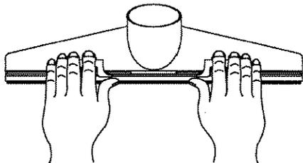
2. Using both hands, position each thumb on the removable insert, (below the latches) and two fingers of each hand on each latch, lift and disengage the two latches from the tabs on the nozzle body.
