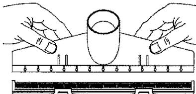
3. Press down with each thumb below the latching tabs until you see and hear the removable insert snap into the nozzle body. Snap the latches over the locking tabs into their original position.
