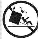
To reduce the risk of tipping, the appliance must be secured by properly installed anti-tip screws provided with the unit. Refer to the Installation Instructions for proper anti-tip bracket installation.
