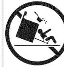
To reduce the risk of tipping, the appliance must be secured by properly installed anti-tip screws provided with the unit. Refer to the Installation Instructions for proper anti-tip bracket installation.
