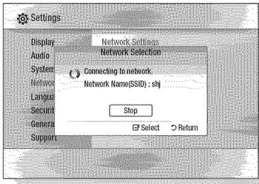
5. In the list of networks, press the ▲▼ buttons to select a network, and then press the ENTER button.
