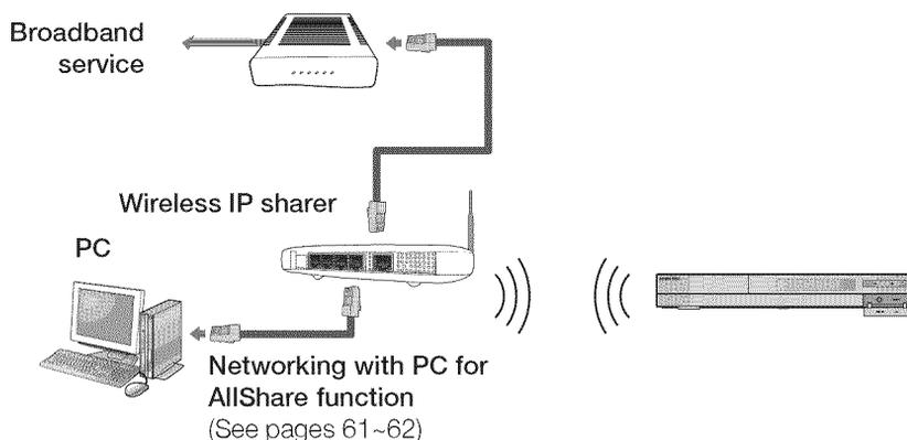
You can connect the player to your network with a Wireless IP sharer. A wireless AP/IP router is required to make a wireless network connection. To set the network options, see page 39.
