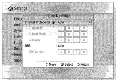
2. After the Network Function has acquired the network values, press the **RETURN** button. Then, run a Network Test to ensure the product has connected to your network (See page 42).
