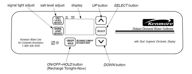
When the transformer is plugged in, the model code SR31, and a test number (example: k10) show in the face plate display for 4 seconds. Then, 12:00 AM and PRESENT TIME begin to flash.
