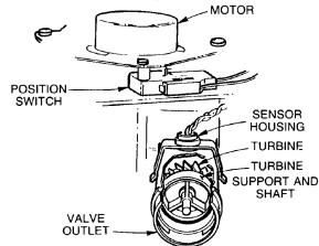
POSITION SWITCH STATUS: WIth the valve in service, or any of the recharge cycles, the switch indicator will show open →. While the valve is rotating from 1 position to another, the indicator will show the switch closed →. A defect is probable if indications vary from this pattern.
