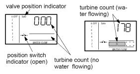
TURBINE OPERATION: If no water is flowing through the softener, the turbine indicator displays 3 zeros. When water is flowing, the flow bar scrolls across the display, and a 000 to 199 count repeats for each gallon of water passing through the turbine. To check for positive operation of the turbine if zeros are shown, open a nearby **soft** water faucet and observe the turbine count and flow bar.
