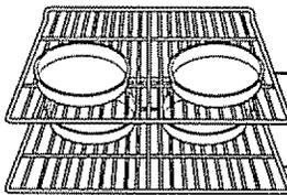
When baking four cake layers at a time, use racks B and D. Place the lower pans at the back of the rack and the upper pans to the front of the rack shown so that one pan is not directly above another.
