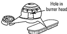
The oval burner head/cap assembly is removable. Simply lift it off the range for cleaning. Use a sewing needle or twist-tie to unclog the small hole in the burner heads.
