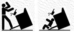
**⚠ WARNING:** If your range is removed for cleaning, servicing or any reason, be sure the anti-tip device is reengaged properly when the range is replaced. Failure to take this precaution could result in tipping of the range and cause injury.
