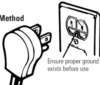
The power cord of this appliance is equipped with a 3-prong (grounding) plug which mates with a standard 3-prong grounding wall receptacle to minimize the possibility of electric shock hazard from this appliance.
