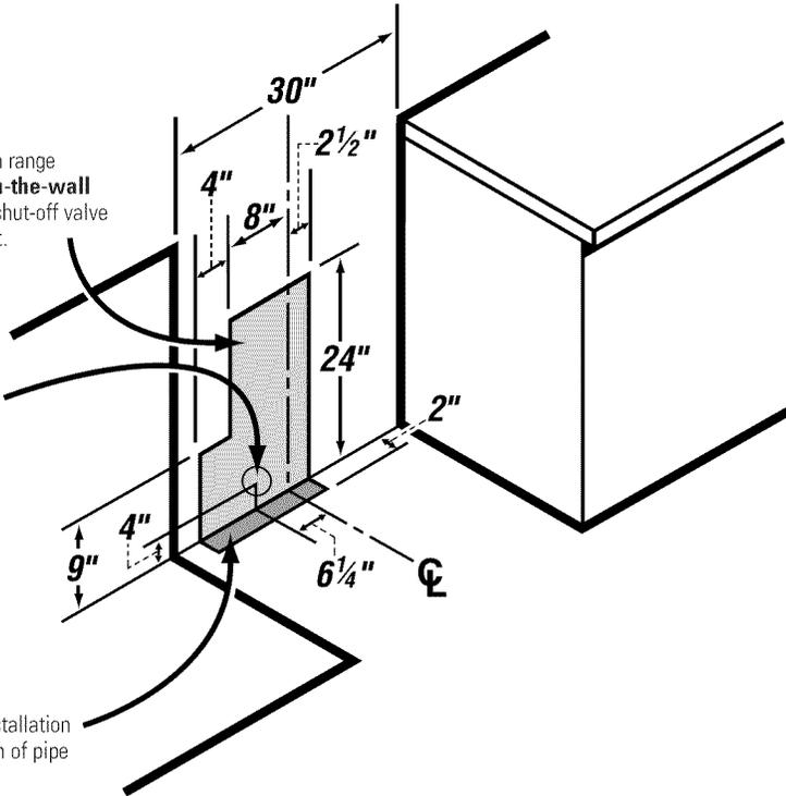
This area allows for flush range installation with **through-the-floor** connection of pipe stub/shut-off valve.
