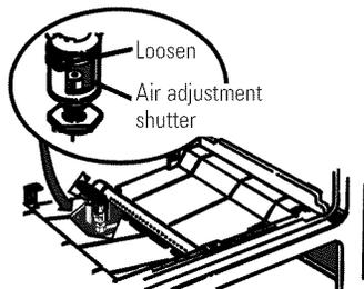
The shutter for the bottom (oven) burner is near the back wall behind the warming drawer, storage drawer or kick panel. Remove the drawer or panel. See the *Care and cleaning of the range* section.
