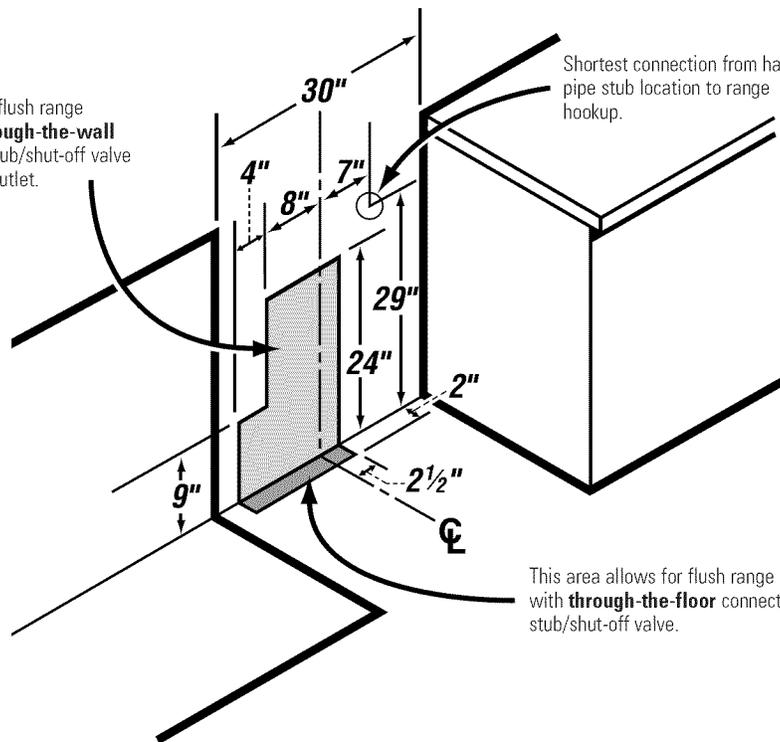
This area allows for flush range installation with **through-the-floor** connection of pipe stub/shut-off valve.
