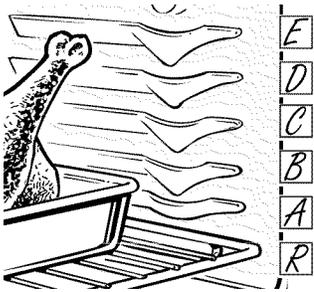
The oven has a special low rack (R) position just above the oven bottom. Use it when extra cooking space is needed, for example, when cooking a large turkey. The rack is not designed to slide out at this position.
