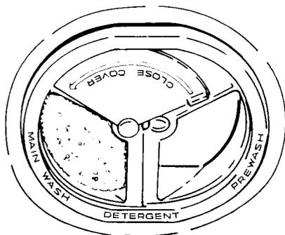
Add detergent to Main Wash compartment for the Light/China Wash Cycle when the dinnerware is lightly soiled.
