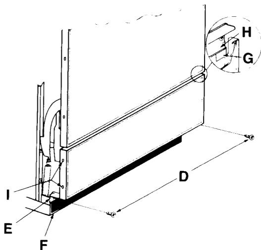
1. Remove two screws (D) located under panel assembly.
