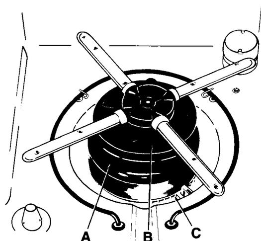
The removable coarse strainer (C) prevents bones, pits and other large objects from entering the pump system. Occasionally check the strainer for such items that may have mistakenly gotten into the dishwasher.
