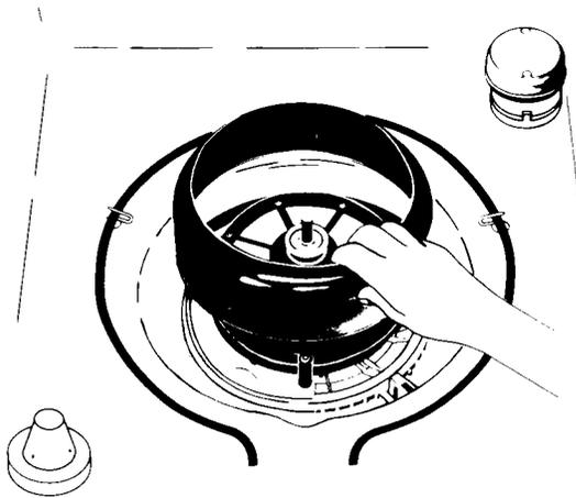
The coarse strainer may be removed, if necessary. To remove, lift strainer out by squeezing center section (F) and remove. To replace, squeeze center section so clips snap into square notch.
