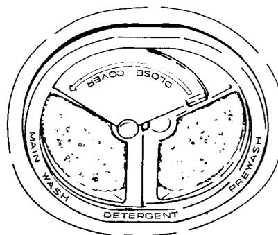
Add detergent to both the Prewash and Main Wash compartments for the Light/China Wash Cycle, the Normal Wash Cycle and the Pots/Pans Cycle when dishes are heavily soiled.
