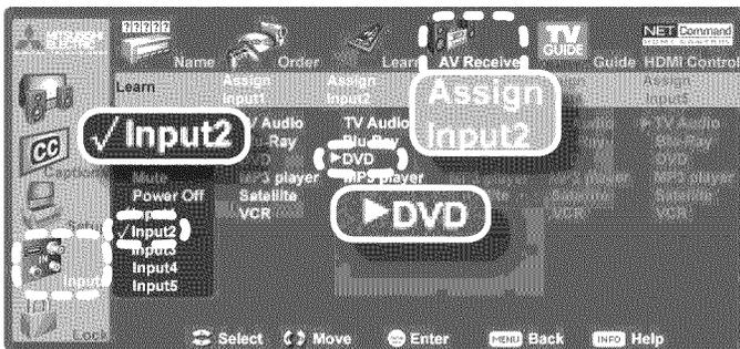
Completed NetCommand setup described for controlling A/V receiver switching to an A/V receiver input "learned" as **Input2**.
