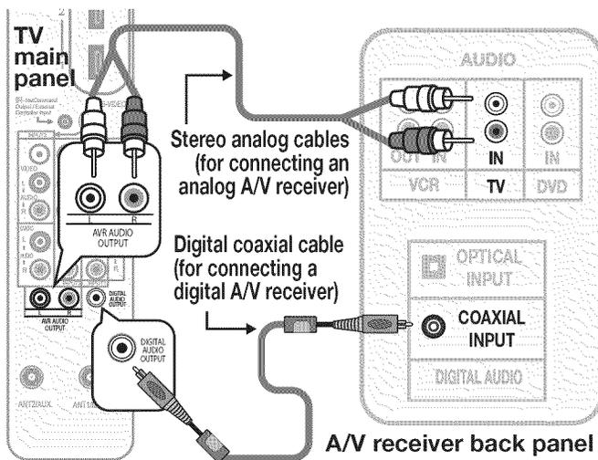
Figure 12. Connecting the TV to an A/V receiver
