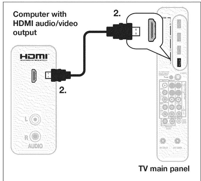
An HDMI-to-HDMI connection carries all video and audio on a single cable.
