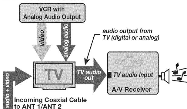
**Audio Switching Setup 1:** Audio to the A/V receiver from the TV's digital or analog audio output
