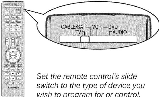
Set the remote control's slide switch to the type of device you wish to program for or control.
