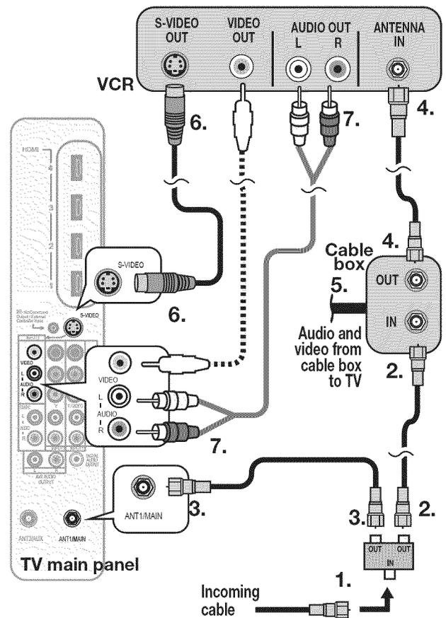
Figure 9. Connecting a VCR to a cable box
