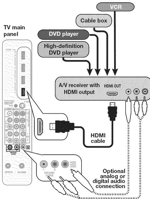
Multiple video inputs on a single HDMI cable. You can connect multiple video devices to an A/V receiver that has an HDMI output. The optional audio connection allows you to hear, through the A/V receiver, devices connected to the TV only.
