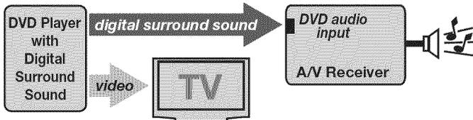
**Setup 2:** A/V receiver audio from a device providing surround sound directly to the A/V receiver
