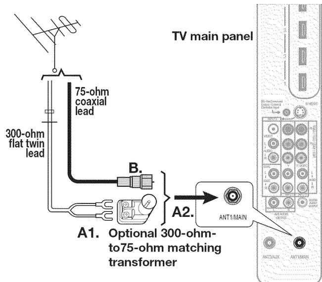
Figure 7. Connecting a Single Antenna Lead
