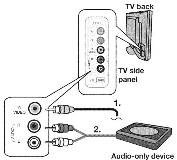
Figure 11. First insert an unused RCA-type connector into the **VIDEO/Y** jack on the TV side or main panel before connecting audio cables.
