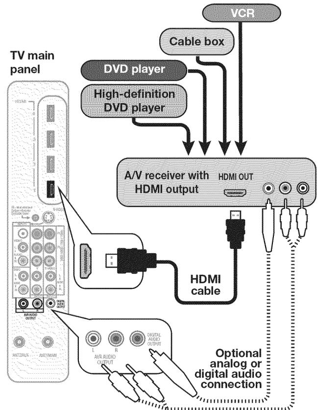
Figure 13. An A/V receiver connected to the TV with an HDMI cable may offer special control capabilities.
