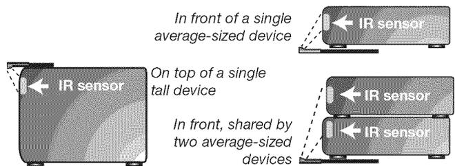
Place IR emitters so the signal can be "seen" by the IR sensor on each device.
