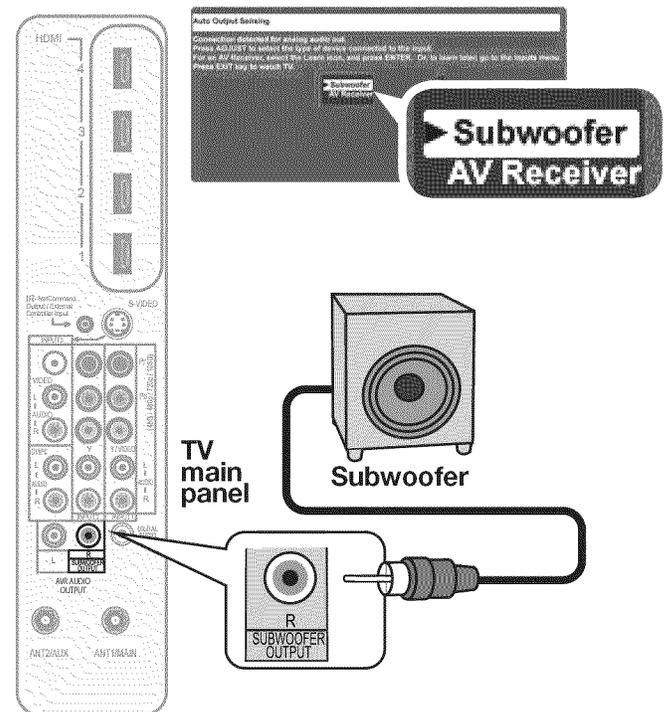
Figure 15. Connecting a subwoofer. When the Auto Output Sensing screen displays, select Subwoofer..
