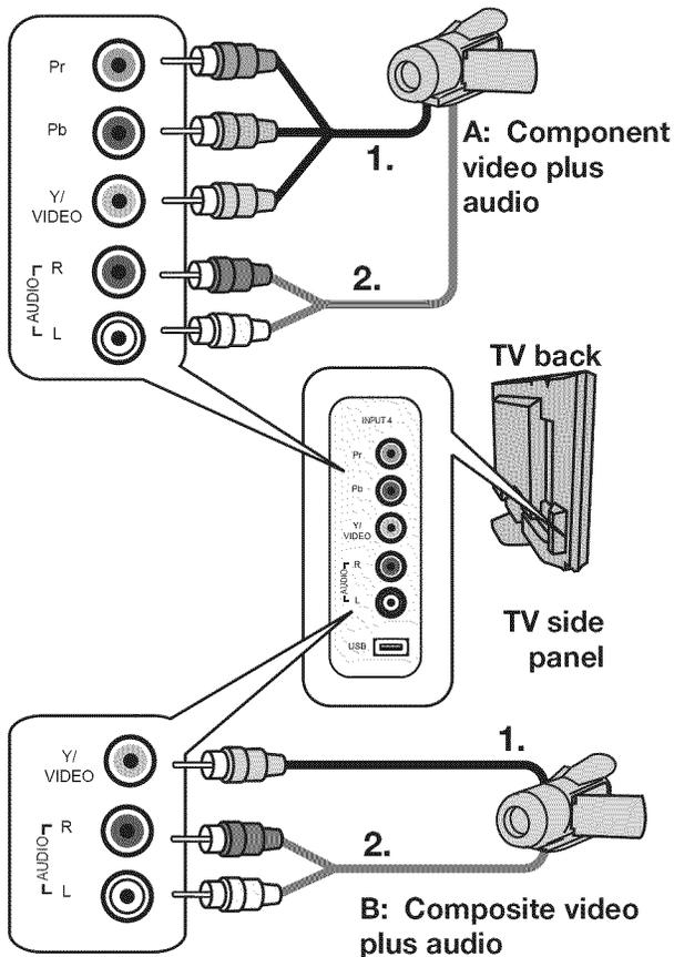
Figure 14. Two connection options for a camcorder.
