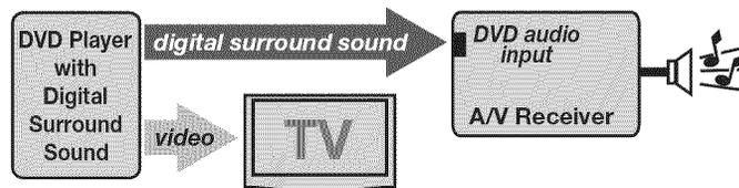
**Audio Switching Setup 2:** Audio from a device providing surround sound is sent directly to the A/V receiver.
