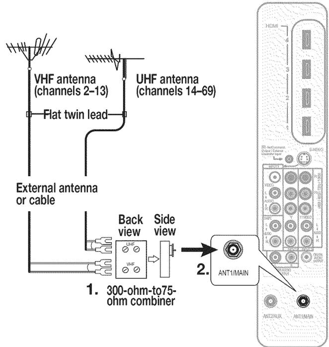
Figure 6. Connecting separate UHF and VHF Antennas
