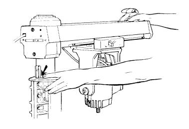
2. Loosen (2)  $^{4}$  – 20 Gib set screws on the left side at the rear of the column support.
