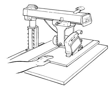
Thus, when standing in front of the saw, the blade would be rotating counterclockwise. After positioning the guard and antikickback mechanism the workpiece is fed from the right-hand side of the saw. The "Blade In-Rip" scale is on the right-hand side of radial arm.
