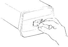
Insert finger under end of switch lever and pull end out, to turn switch on.
