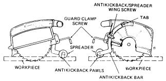
Make sure by trial — without saw running — before starting the cut that the antikickback pawls will stop a kickback once it has started. Insert workpiece alongside spreader under outer set of pawls by approaching pawls in the feed direction. Push workpiece sharply in the direction of a kickback (opposite to direction of feed). Readjust Pawls if they do not stop the kickback motion by biting into the workpiece.
