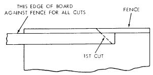
Turn workpiece over end for end . . . keep same edge against fence when making successive cuts.
