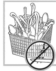
Do not let any item extend through the bottom of the silverware basket. Items that extend through the rack could prevent the spray arm from turning and cause poor wash performance.
