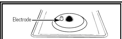
The electrode of the spark igniter is exposed when the burner head is removed. When one burner is turned to **LITE**, all the burners spark. Do not attempt to disassemble or clean around any burner while another burner is on. An electric shock may result, which could cause you to knock over hot cookware.
