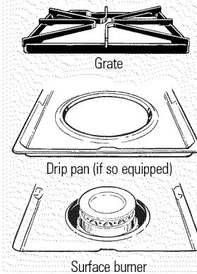
**CAUTION:** Do not operate the cooktop without all burner parts, drip pans (if so equipped) and grates in place.
