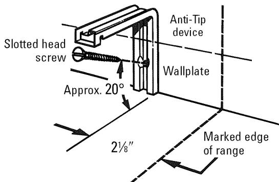
B. Locate the outside edge of the device  $2\frac{1}{8}$ " toward the center of the range from the marked edge of the range.
