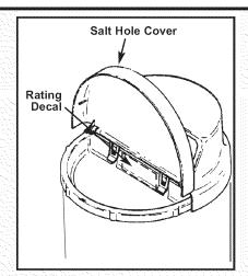
\* The model number is on the rating decal, located on the rim, under the salt hole cover.
