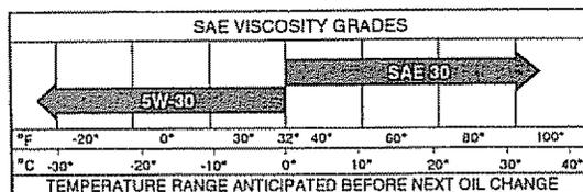
**NOTE:** Although multi-viscosity oils (5W30, 10W30 etc.) improve starting in cold weather, these multi-viscosity oils will result in increased oil consumption when
