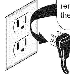
Power supply cord with 3-prong grounding plug
