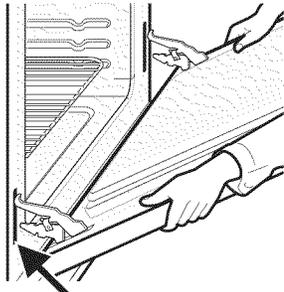
HINGE SLOT - Door removed
