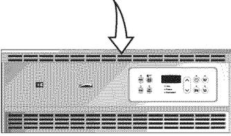
**CAUTION** Some models are equipped with a blower which runs in baking and self-cleaning mode to keep all internal components at a cool temperature. The blower may keep running even if the oven has been turned off, until the components have cooled down.
