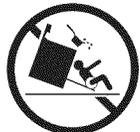
To reduce the risk of tipping, the wall oven must be secured by properly installed mounting brackets provided with the wall oven. Refer to the Installation Instructions for proper mounting bracket installation.
