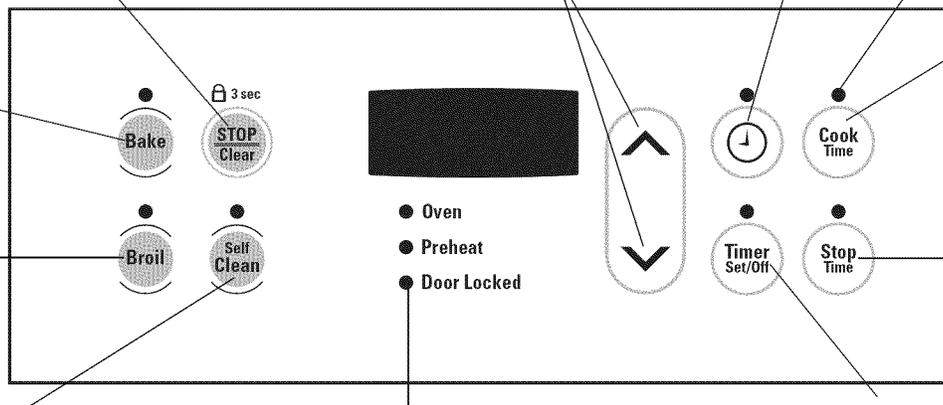
\*Note: The **OVEN** indicator light on the electronic display will turn ON and OFF when using the Bake feature and during preheat. This is normal and indicates that the oven is cycling to maintain the selected baking temperature. When the preheat indicator light turns OFF, your oven is ready.
