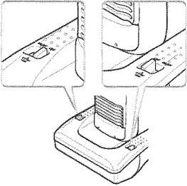
The E-Z Belt Check consists of two latches on the top of the floor nozzle. These latches allow for easy removal of the nozzle cover to change the belt or clean the agitator.
