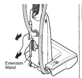
Remove the extension wand from its storage position.
