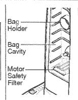
Check the bag holder and the motor safety filter.
