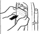
Insert the dust bag onto the bag holder completely by holding the bag collar as shown and snapping it into position.
