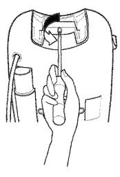
Position the handle as shown below and slide the handle into the opening at the top of the vacuum.
