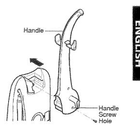
Tighten the screw securely with a screwdriver. It may be necessary to adjust the handle
