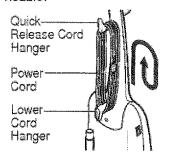
Wrap the power cord around the quick release cord hanger and lower cord hanger, and clip the plug onto the power cord.
