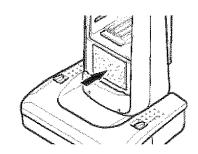
Carefully replace the dust cover by placing tabs in slots and pushing in until cover snaps into place.
