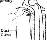
Pull the dust cover forward. Remove and lay aside.
