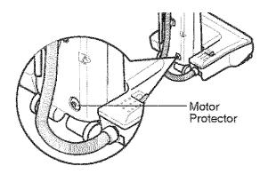
To correct problem: Check for and remove clogs. See CLOG REMOVAL.
