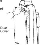
Grasp the dust bag collar and pull gently, carefully removing the dust bag.
