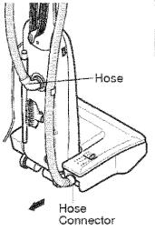
Re-insert the hose into the opening on the lower body from which it was removed. Press firmly to assure connection.
