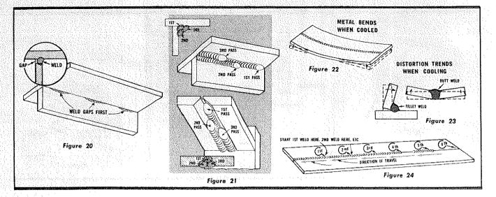
To simulate actual conditions tack-weld a piece with an irregular edge to another piece leaving numerous gaps along the joint. Use the whipping motion and deposit a fairly heavy bead, slowing down the rate of travel where the gaps are widest to build up a weld of uniform size throughout its length. If the gaps are rather wide, fill them first, clean off the slag and lay in a fillet weld the entire length of the joint (fig. 20).
