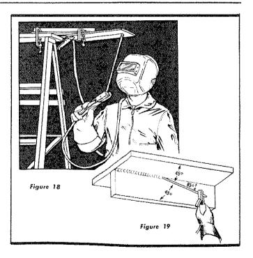
Fillet welds for lap or tee-joints are most common in the overhead position. Tack-weld two pieces of scrap iron together to form a tee-joint, and clamp in the overhead position so one plate is held vertically (fig. 19). Hold the rod at angles indicated and deposit a light bead from left to right without weaving or whipping movements. A slightly higher current than used for overhead butt welds will be necessary to get good penetration at the root of the weld.
