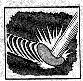
Figure 4 Watch the weld puddle to keep the slag from flowing in front of it, causing inclusions and gas pockets.
