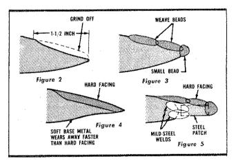
must be deposited along the edge to build it up (fig. 3). Make beads heaviest where the wear will be greatest, but avoid excessive build-up as the metal cannot be filed or machined. If shaping is required, heat the weld metal and forge it. Smoothing and sharpening can be accomplished by grinding.
