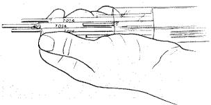
Now loosen the heat selector knob and move the pointer until the fractional number matching your electrode diameter appears in the pointer window.
