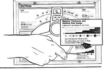
C. Finally, determine the type of electrode by the identification on the package or by the American Welding Society number stencilled on the coated portion of the electrode, bearing in mind the type of electrode you have chosen — E6013 or E7014, and also its' diameter (as previously determined).
