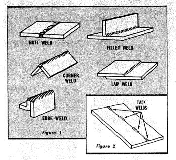
Flat welding includes all types of joints in which the weld is horizontal, and the electrode is fed down as in the practice welds of previous pages. The five types of joints in figure 1 can be welded in the flat position.
