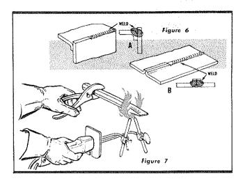
aluminum alloy, use aluminum flux. The filler rod should be of the same analysis as the work. If regular welding rod is not available, strips of the parent metal may be used. A back-up strip should be used when welding thin material.
