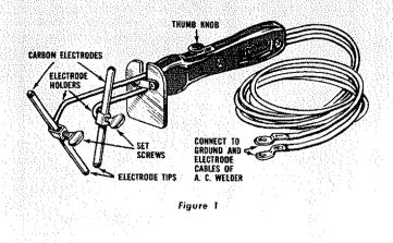
Work ordinarily done with a gas welding torch is possible with the twin-carbon arc torch connected to an A.C. welder. The carbon-arc flame is similar to the flame of a gas welding torch in that it provides heat by radiation, rather than by direct arc between work and electrode. This flame heat greatly widens the scope of work possible with the arc welder for brazing, soldering, welding of non-ferrous metals and localized heating for bending, forging and hardening.
