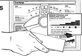
B. Next verify the electrode diameter, by placing the bare portion of the electrode against the electrode diameter gauge located under the bar chart.
