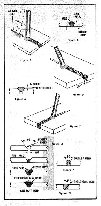
over and weld a similar bead on the other side (fig. 7). A higher welding current can be used on this side as there is no danger of burning through and fusion with the first bead will be assured.
