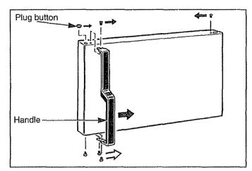
(a) Remove screw holding handle to top of door.
