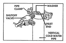
**5.** Fasten shutoff valve to cold water pipe with pipe clamp. Be sure inlet end is solidly in 3/16" drilled hole in water pipe and washer is under pipe clamp. Tighten packing nut. Tighten pipe clamp screws carefully and evenly so washer makes a watertight connection. Do not overtighten or you may crush copper tubing, especially if soft copper tubing is used. Now you are ready to connect the copper tubing.
