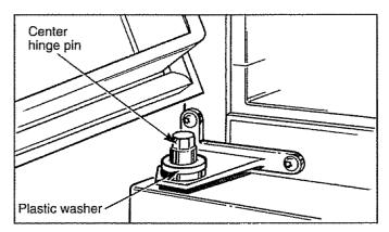
(a) Lower the bottom socket of the freezer door onto the center hinge pin. Be sure the washer is in place.
