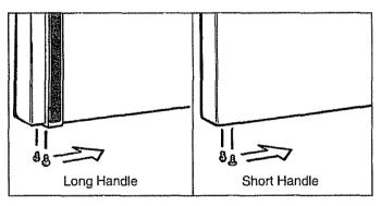
(a) Transfer two screws in bottom left of door to opposite side. (Wait until handle is moved before reinstalling front screw.)
