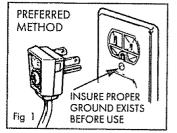
Have wall outlet and circuit checked by a qualified electrician to make sure outlet is properly grounded.
