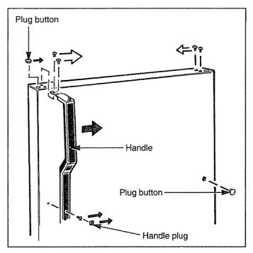
(b) Remove two screws holding handle to top of door.
