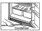
accessible on condenser coils, then turn the control back on. For best results, use a brush specially designed for this purpose. It is available at your Sears store or service center. This easy cleaning operation should be done at least once a year.
