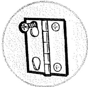
2 Loosen top screw from each hinge on the dryer face half way. With one hand holding the top of the door and the other hand holding the bottom, remove the door from the dryer by lifting it **UP** and **OUT**.
