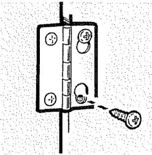
4 Remove the remaining screws from the side of the opening from which the door was removed. With these screws secure each hinge at the bottom. Tighten the two top screws of each hinge. Reinsert the plastic plugs on the side from which the door was removed.
