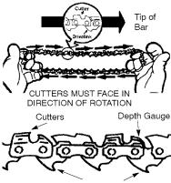
Drive Links 8. Place chain over and behind clutch, fitting the drive links in the clutch drum sprocket.
