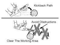
A WARNING: Avoid kickback which can result in serious injury. Kickback is the backward, upward or sudden forward motion of the guide bar occurring when the saw chain near the upper tip of the guide bar contacts any object such as a log or branch, or when the wood closes in and pinches the saw chain in the cut. Contacting a foreign object in the wood can also result in loss of chain saw control.
