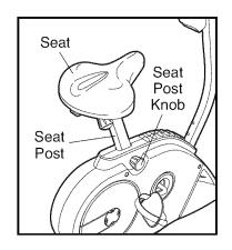
slide the seat post upward or downward to the desired position, and then release the knob. Move the seat post upward or downward slightly to make sure that the knob is engaged in one of the adjustment holes in the seat post. Then, tighten the knob.
