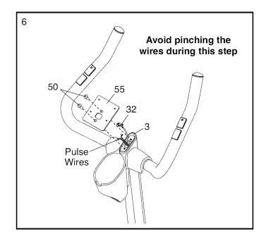
7. While another person holds the Console (6) near the Upright (3), connect the console wires to the Upper Wire Harness (32) and to the pulse wires.
