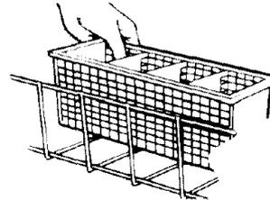
Load the silverware basket while it's in or out of the bottom rack. The loaded basket should be in the right front corner of the bottom rack.
