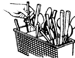
Make sure sharp items (knives, forks, skewers, etc.) are put in point down. Make sure long items do not stop the upper spray arm from turning.
