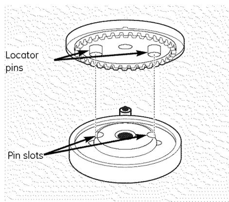
When replacing, make sure the locator pins in the burner head are seated in the pin slots of the burner base. Rotate the burner head around the burner base until it is level and securely seated.
