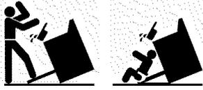
If your range is removed for cleaning, servicing or any reason, be sure the anti-tip device is re-engaged properly when the range is replaced. Failure to take this precaution could result in tipping of the range and cause injury.
