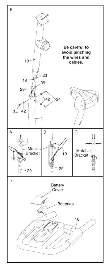
8. While a second person holds the Console (16) near the Upright (13), connect the console wire to the Extension Wire (23). Then, insert the wires downward into the Upright.
