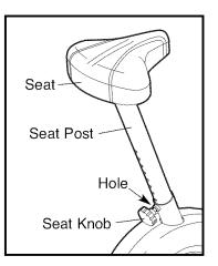
slide the seat post upward or downward and align one of the adjustment holes in the seat post with the indicated hole in the Frame. Insert the seat knob into the frame and the seat post, and turn the seat knob clockwise until it is tight. Make sure that the seat knob is inserted through one of the adjustment holes in the seat post.
