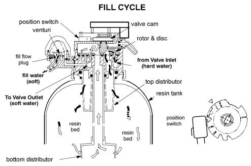
To begin a regeneration, the electronic timer energizes the circuit to the valve motor. The valve motor rotates the rotor and disc and the valve cam until the position switch drops, to open the motor circuit and position the valve in FILL. As the rotor and disc rotates, the port opens for SOFT water fill through the venturi. Fill flow continues to the brine valve, and into the salt storage tank. Soft water is still available to the house lines.
