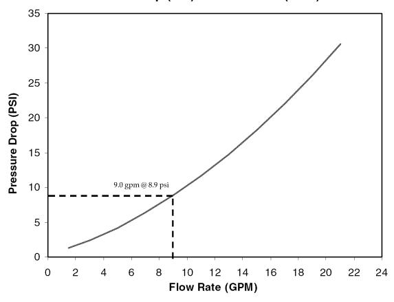
Intermittent flow rate does not represent the maximum service flow rate used for determining the softeners rated capacity and efficiency. Continuous operation at flow rates greater than the service flow rate may affect capacity and efficiency performance.
