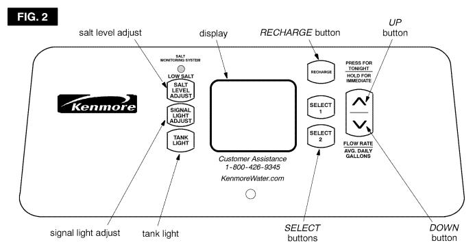
When the transformer is plugged in, the model code HF36, and a test number (example: J1.0) show in the face plate display for 4 seconds. Then, 12:00 AM and PRESENT TIME begin to flash.
