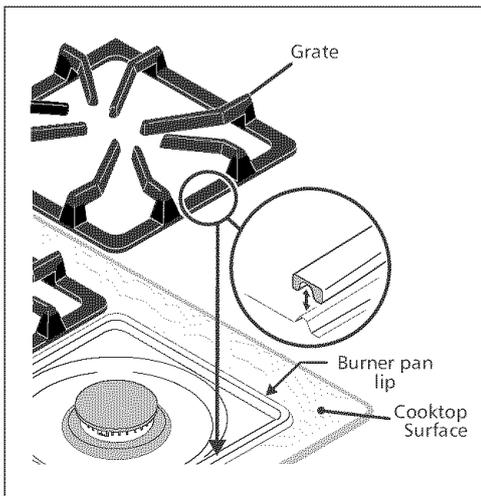
Place grate over burner pans. Make sure that the groove under grate fits over the raised lip of the burner pan. The rounded corners of the grates should be placed toward the front of the cooktop for the front burners and the rear of the cooktop for the back burners.
