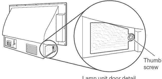
4. Using a manual Phillips screwdriver, loosen the two screws on the lamp unit.
