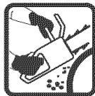
Never operate a chain saw holding it with one hand only.
