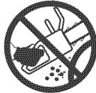
Contact of the guide bar tip with any object must be avoided.
