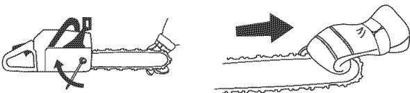
The position of the chain tensioning screw on our chain saws varies from model to model. See instructions under the heading What is what? to find out where it is on your model.
