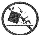
To reduce the risk of tipping, the wall oven must be secured by properly installed mounting bracket provided with the wall oven. Refer to the Installation Instructions for proper mounting bracket installation.
