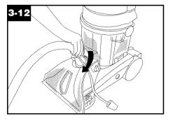
Insert short hose end, matching tabs on hose with same-sized slots in port.
