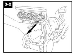
d. Remove lint from filter screen located on bottom of cleaner as follows.
