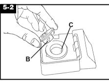
3. Align slots (B) on cap with tabs (C) in opening.
