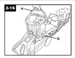
Turn recovery tank latches (G) outward (one on each side of tank).
