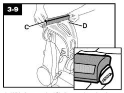
2. With foam strip (C) (located under the netting) in position as shown, place attachment on front of nozzle (D). Make sure arrow on end of attachment points in the direction as shown.
