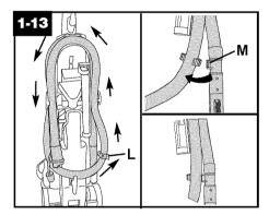
Loop hose over top of caddy again. Slide hose clip (L) toward end of hose. Snap tab (M) on hose connector into hose clip.
