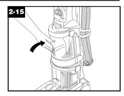
Position bottom of tank onto cleaner and pivot tank to snap it into place.
