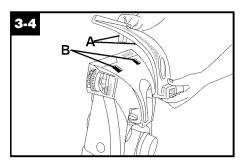
To replace nozzle, line up tabs (A) on nozzle with holes (B) in cleaner. Slide tabs into holes.
