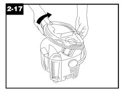
Lower handle toward back of tank to unlock lid. Lift lid off tank. Empty tank and reposition lid.
