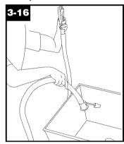
Drain solution tube by placing round end in sink and raising nozzle above your head. Press the trigger.
