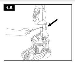
Push bolts into holes on front of handle. If bolts will not go through hole easily, handle is not pushed completely down.
