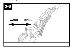
10. For best results, use straight, parallel strokes as shown in the diagram below. Overlap strokes by 1 inch to help prevent streaking.
