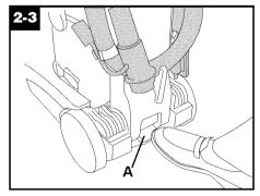
Handle release pedal Step on pedal (A) to lower handle to operating position. Handle does not lock into a single position but "floats" to allow convenient operation.
