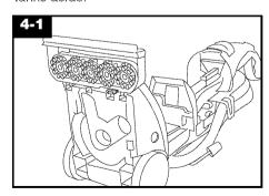
With handle in upright position, tilt cleaner back until handle rests on the floor.
