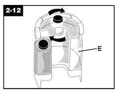
Fill tank (E) (1 gallon) with hot tap water. CAUTION: Do not fill with water above 140°F (60°C).
