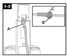
NOTE: If the cord protector (A) on back of handle should become dislodged during unpacking, make sure it is repositioned properly before continuing with assembly of your deep cleaner. With the arrow (B) on the cord protector pointing down, press groove (C) in the cord protector into slot in the lower handle.
