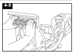
Grab brush assembly and pull firmly. The brushes can be cleaned under running water.
