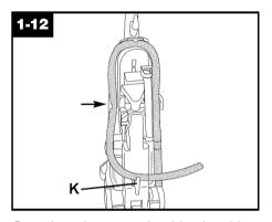
Press hose into opposite side of caddy. Loop hose at bottom of cleaner and press into top of hook (K).
