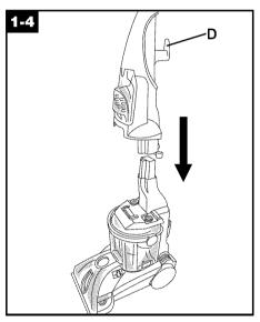
With cord hook (D) to back of deep cleaner, push upper handle down onto lower handle.
