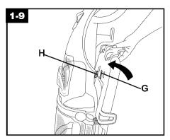
Rotate top of caddy toward cleaner handle. Slide caddy down so notch (G) on caddy rests in hook (H) on cleaner.
